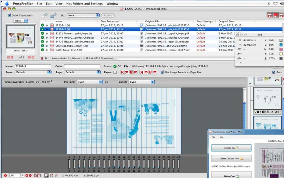
Press Profiler is a powerful and easy to use ink coverage and ink zone calculation solution for offset printing presses providing ink key presetting for a faster make-ready and reduced consumables cost.
